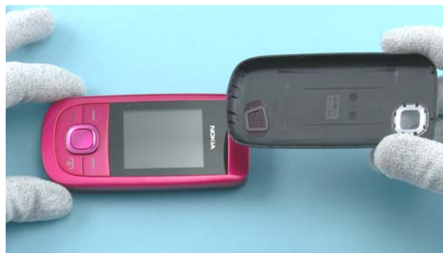
4) Remove the BATTERY COVER. If there is a battery inserted, remove it also.
