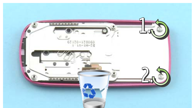
18) Unscrew the two TORX+ size 4 screws in the order shown. Do not use them again. Discard them.
