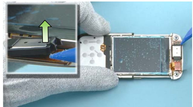
24) Using the sharp end of the SS-93, lift up the EARPIECE HOLDER.
