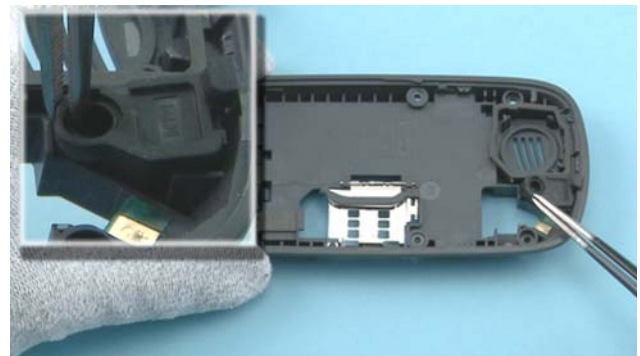
12) Use the tweezers to remove the MIC RUBBER FRAME from the D-COVER.
