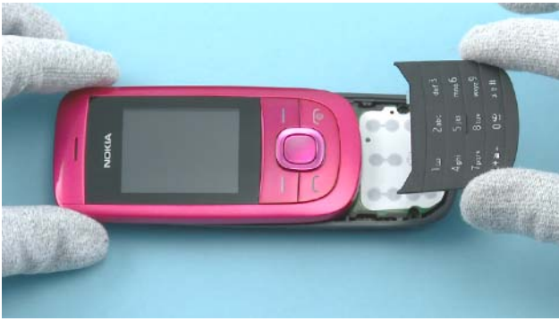
7) Remove the NUMERICAL KEYMAT ASSY.
