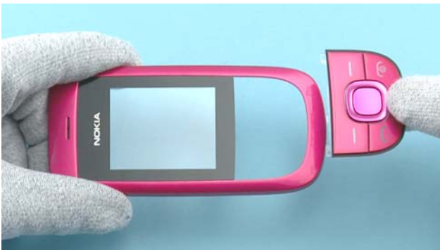
23) Remove the FUNCTIONAL KEYMAT ASSY.
