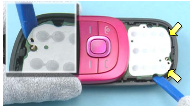
8) Using the SS-93, detach the two clips holding the SLIDER MODULE.
