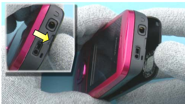
3) Use the opening notch to release the BATTERY COVER.
