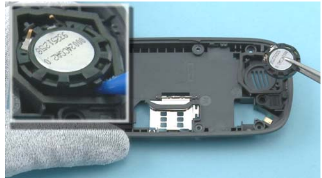
10) Lift up the IHF SPEAKER with the sharp end of the SS-93. Remove the IHF SPEAKER.
