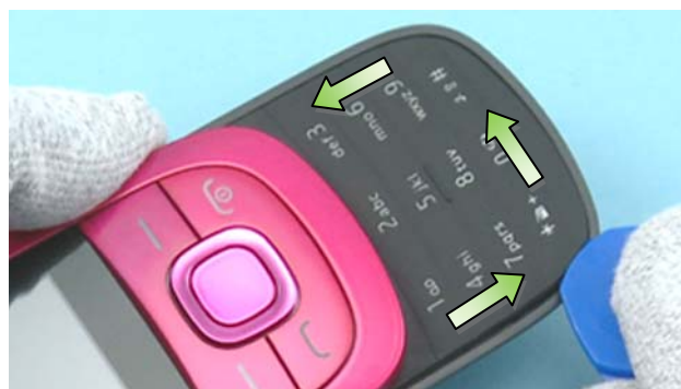
6) Insert the SRT-6 between the NUMERICAL KEYMAT ASSY and the D-COVER. Slide the SRT-6 in the direction shown.
