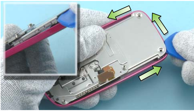
19) Slide the SRT-6 between the SLIDER MODULE and the A-COVER in the direction shown.
