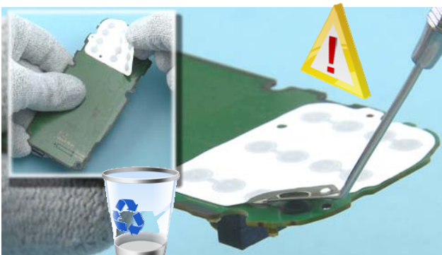
17) Use the dental tool to lift up one corner of the DOMESHEET. Peel off and remove the DOMESHEET ASSY with fingers. Do not use it again. Discard it. Be aware of the sharp point of the dental tool – be careful not to injure yourself!
