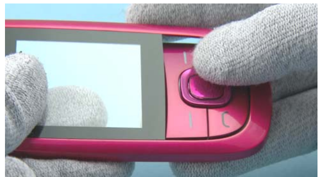
22) Detach the FUNCTIONAL KEYMAT ASSY from the A-COVER by pressing it down.
